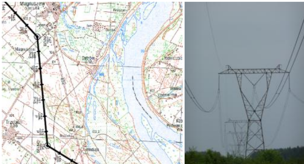
Figure 9 Plan view of tension section 147-154 of the 400 kV Kozenice – Miłosna power transmission line
